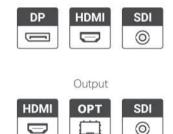
HDR Master supports flexible interface choices, includes: one swappable input card: DP1.2×1, HDMI2.0×1, 12G-SDI×4 and two swappable output cards: one contains HDMI2.0×1, 10G optical fiber×4 and one contains HDMI2.0×1, 12G-SDI×4.
