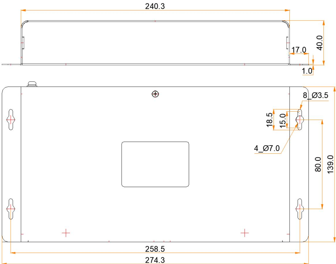
Tolerance:  $\pm 0.3$  Unit: mm
