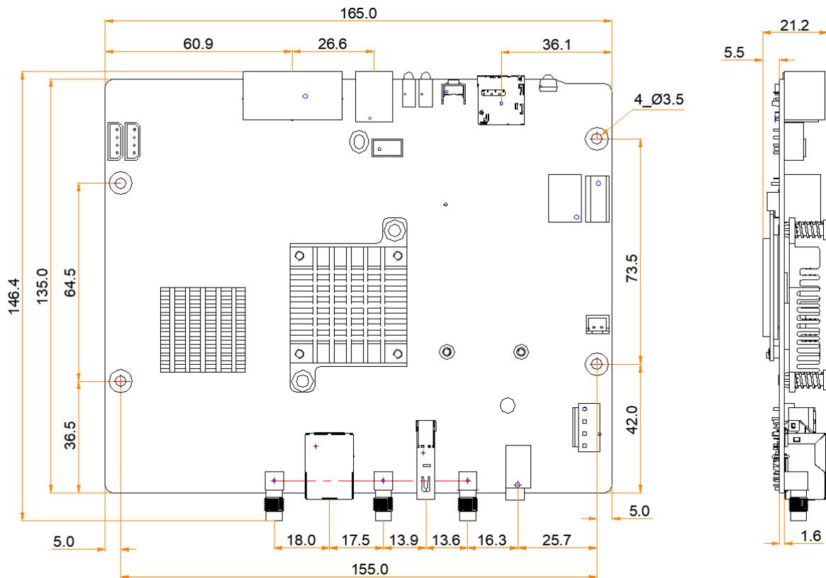
Tolerance:  $\pm 0.3$  Unit: mm
