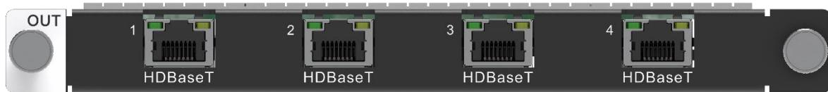
4x RJ45 Gigabit Ethernet ports
